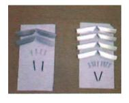
**STEP 3:** Insert galvanized steel corner gusset(s) into end of arch top header, one (1) each for 5 1/2" jamb and two (2) each for 7 1/2" jamb. Gussets should be inserted up to dimple stop in cavities that alian with black dot on back of arch top header.
